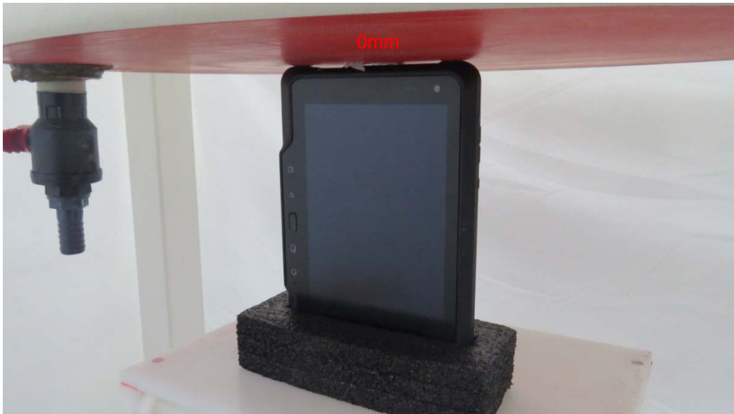
Picture 3: Left Side, the distance from handset to the bottom of the Phantom is 0mm
