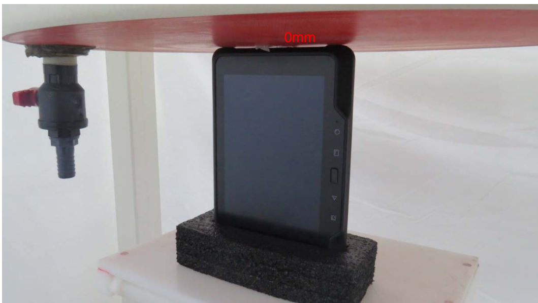
Picture 4: Right Side, the distance from handset to the bottom of the Phantom is 0mm
