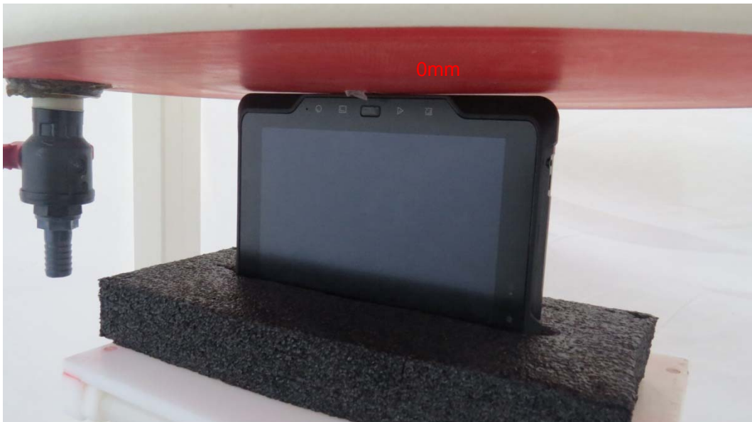
Picture 6: Bottom Edge, the distance from handset to the bottom of the Phantom is 0mm
