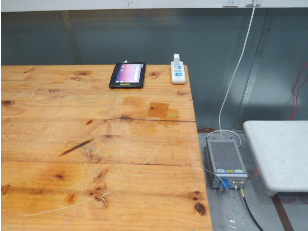
Picture 2 Conducted Emission Test Setup
