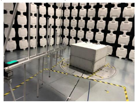
Description: Radiated Emission Test Setup
