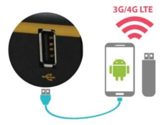
For increased WAN diversity, plug in a USB LTE modem as backup. Peplink routers are compatible with over 200 modem types. You can also tether to smartphones running Android 4.1.X and above.
