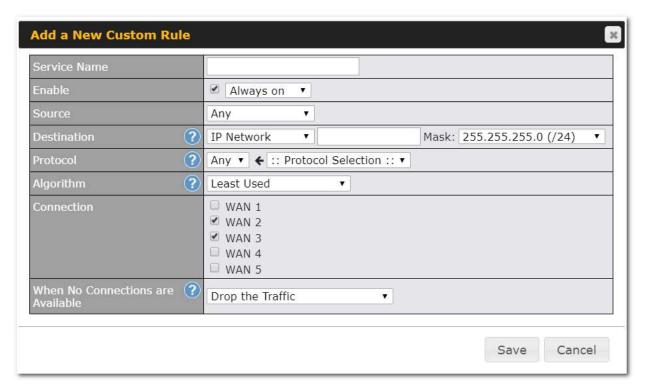
The traffic matching this rule will be routed through the healthy WAN connection that is selected in **Connection** and has the most available download bandwidth. The available download bandwidth of a WAN connection is calculated from the total download bandwidth specified on the WAN settings page and the current download usage. The available bandwidth and WAN selection is determined every time an IP session is made.
