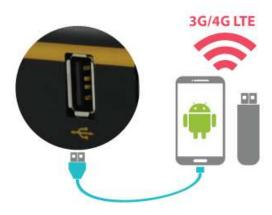
For increased WAN diversity, plug in a USB LTE modem as a backup. Peplink routers are compatible with over <u>200 modem types</u>. You can also tether to smartphones running Android 4.1.X and above.
