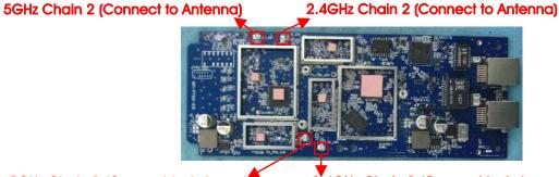
5GHz Chain 1 (Connect to Antenna)
