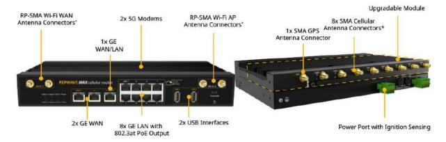
\*For the best performance and reliability, all RF connectors must be connected to the same type and performance antennas.
