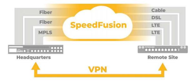
Pepwave bandwidth bonding SpeedFusion<sup>™</sup> is our patented technology that enables our SD-WAN routers to bond multiple Internet connections to increase site-to-site bandwidth and reliability. SpeedFusion functionality securely connects your Pepwave router to another Pepwave or Peplink device (Peplink Balance 210/310/380/580/710/1350 only). Data, voice, or video communications between these locations are kept confidential across the public Internet.
