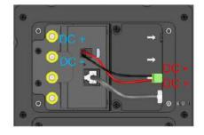
• STEP 6: Lock the slot cover with 4 pcs M3 screws.
