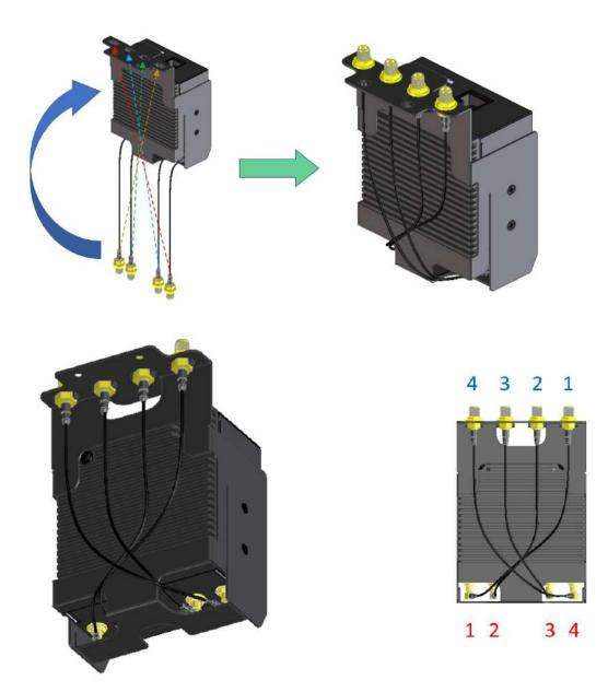
• STEP 4: Lock the SFE-Duo set in the slot with 2 pcs M3 screws.
