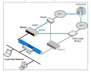
In the diagram, the WAN ports of each Pepwave router connect to the router and to the modem. Both Pepwave routers connect to the same LAN switch via a LAN port.
