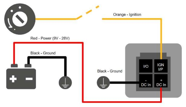
Connectivity diagram for devices with terminal block connection
