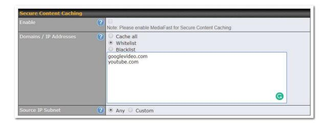
The **Secure Content Caching** menu operates identically to the **MediaFast** menu, except it is for secure content cachting accessible through https://. In order for Mediafast devices to cache and deliver HTTPS content, every client needs to have the necessary certificates installed\*.
