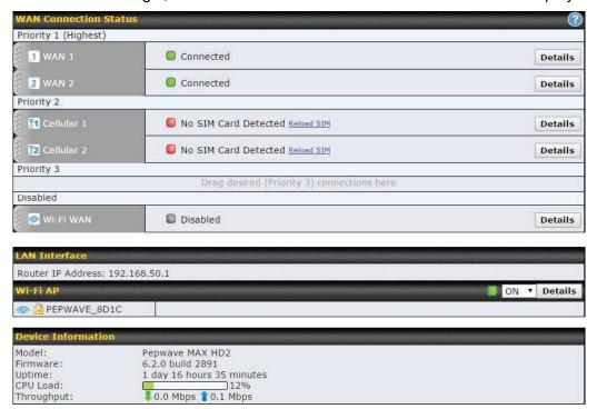
The **Dashboard** shows current WAN, LAN, and Wi-Fi AP statuses. Here, you can change WAN connection priority and switch on/off the Wi-Fi AP. For further information on setting up these connections, please refer to **Sections 8** and **9**.
