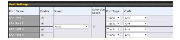
On this screen, you can enable specific ports, as well as determine the speed of the LAN ports, whether each port is a trunk or access port, can well as which VLAN each link belongs to, if any.
