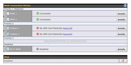
To able a particular WAN connection, drag on the appropriate WAN by holding the left mouse button, move it the **Disabled** row, and drop it by releasing the mouse button.
