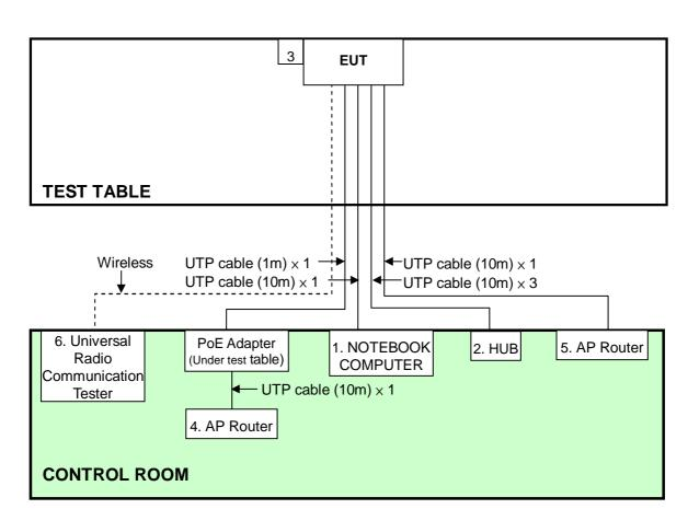
NOTE: 1. Supply unit 3 is the 3.5G USB WIRELESS DEVICE.
