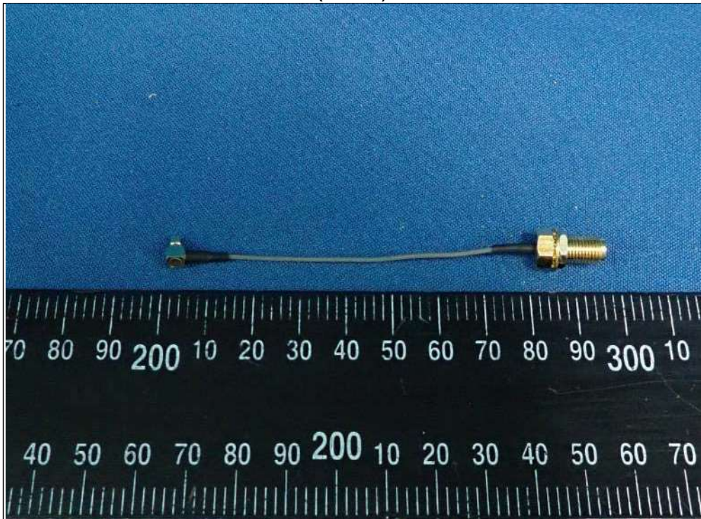
Cellular 2 (Main) Ant. cable
