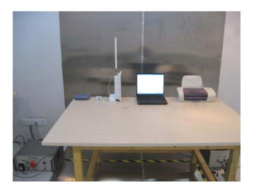
Radiation Emission Test Setup (Below 1GHz)
