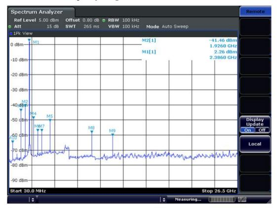
$\label{eq:midchannel} Mid \ channel$   $Frequency \ Range = 30 \ MHz \sim 10^{th} \ harmonic.$
