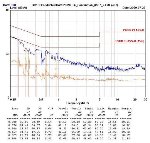
Remarks: C.F (Correction Factor) = Insertion loss + Cable loss
