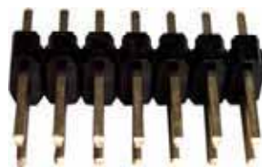
<Figure 7-1-12-④ 2.54mm(100mil) 7*2 Pin Headers >
