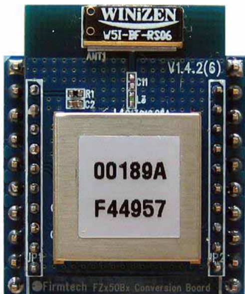
< Figure 7-1-12-⑩ 2.54mm(100mil) Mounting Convertible Board >
