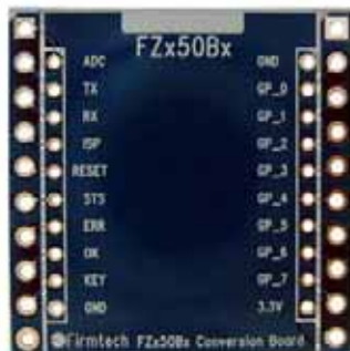
< Figure 7-1-12-⑧ 2.54mm(100mil) A Convertible Board >
