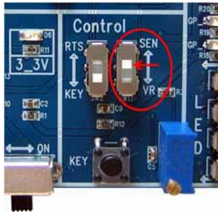
< Figure 7-1-12-② Set-up for use ADC Port as Extension Port >
