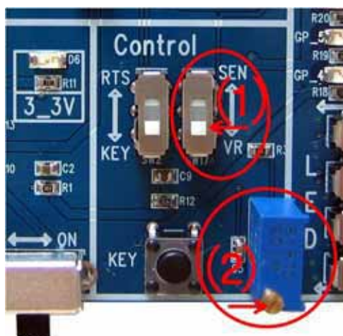
< Figure 7-1-6 Setting VR / SEN Selection Switch to SEN & ADC Data Input Variable Resistance >
