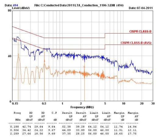
Remarks: C.F (Correction Factor) = Insertion loss + Cable loss
