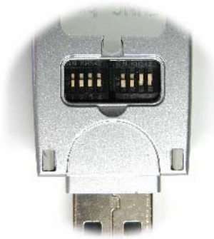
<Figure 5-1 FB200AS Dip Switch View>
