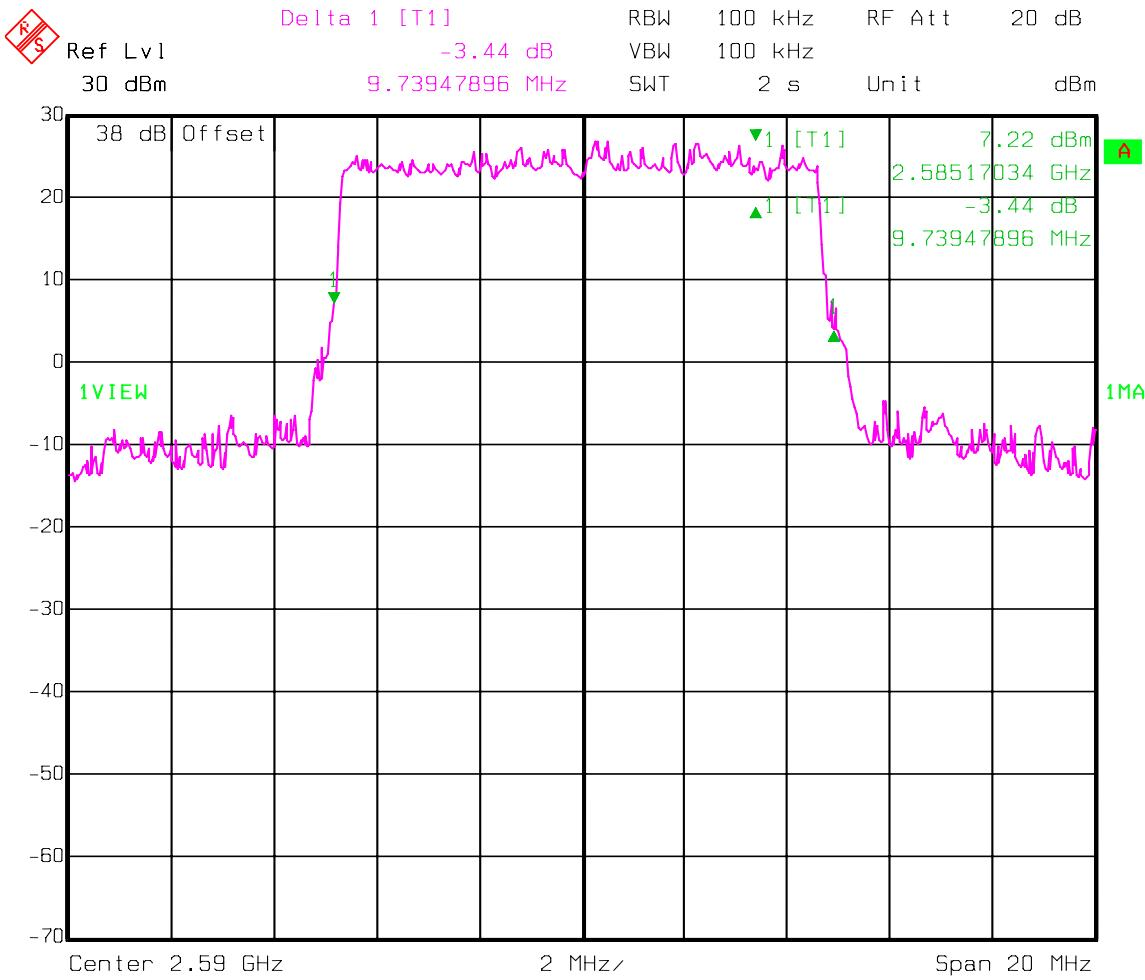
**Occupied bandwidth was identical for all frequencies and modulation types.**
