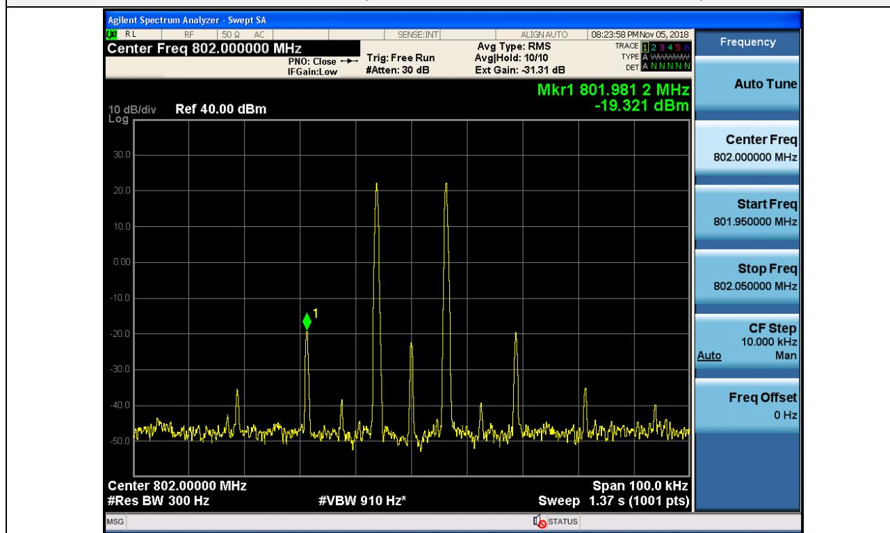
3 dB above the AGC threshold Output Intermodulation / PS Narrowband / Uplink / 6.25 kHz
