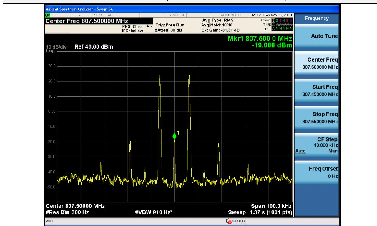
3 dB above the AGC threshold Output Intermodulation / PS B/ILT SMR / Uplink / 25 kHz
