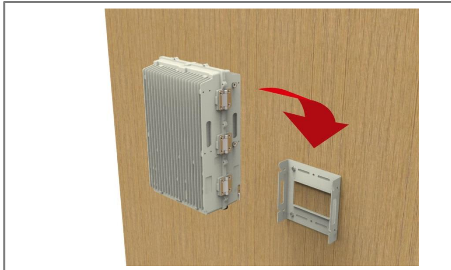
Figure 25. The way to hang the system for Wall Mounting
