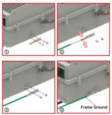
• The specification of ground terminal lug is like below (Refer to JOCT 0202-RL05)
