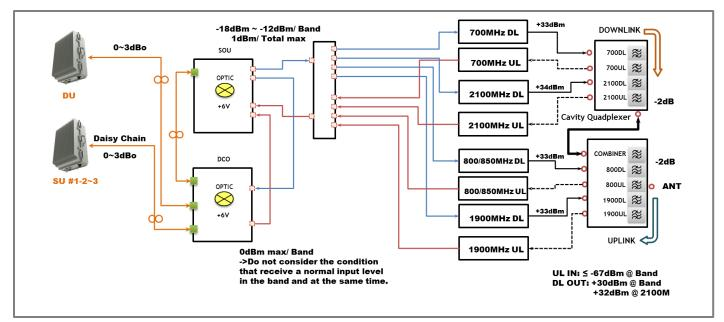
Figure 12. EZS-LICPA30 Block Diagram Configuration
