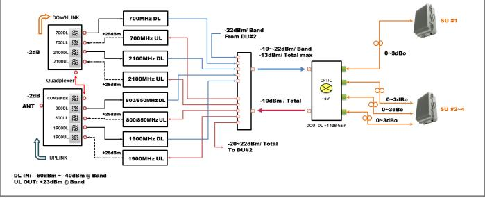
Figure 11. EZD-LICPA23 Block Diagram Configuration
