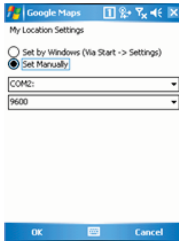
Set the COM Port and Baud Rate.
