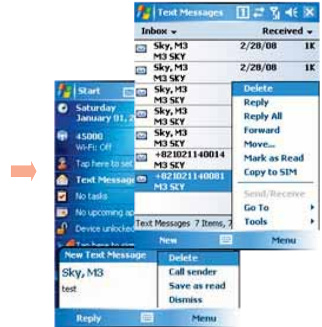
Controlling received SMS can be done by using the menu on the 'New Text Message' alert window or on the Text Messages program.
