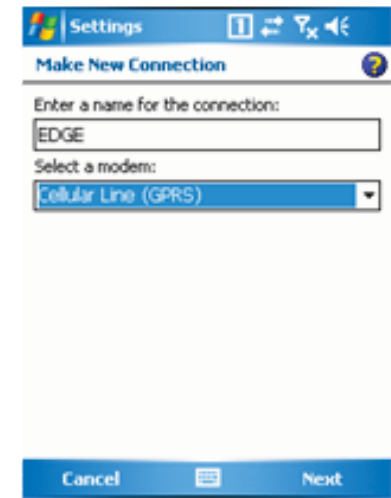
Put the name you want into the 'Enter a name for the connection'. Then select the 'cellular Line(GPRS)' in the 'Select a modem'.
