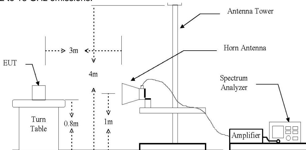
The diagram below shows the test setup for substituted method
