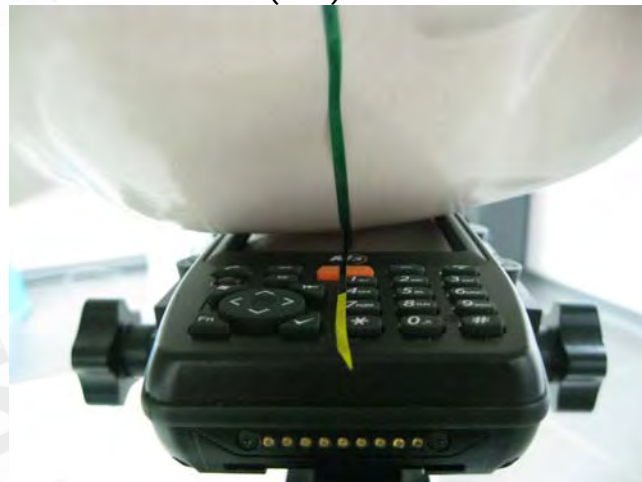
Fig.5 Left Head Section / Cheek-Touch Position
