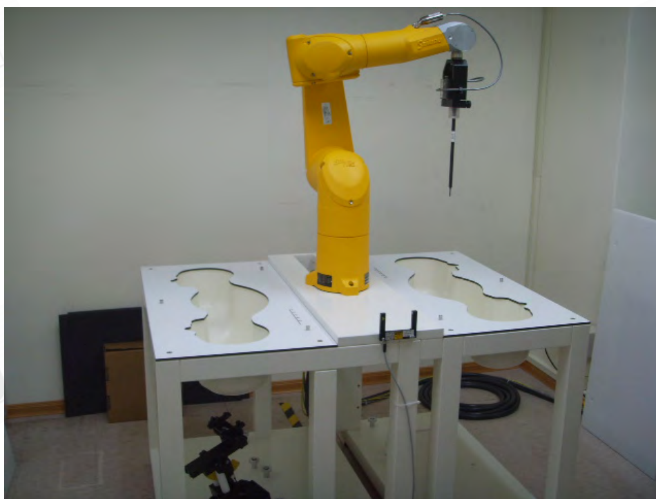
Fig.1 Photograph of the SAR measurement System
