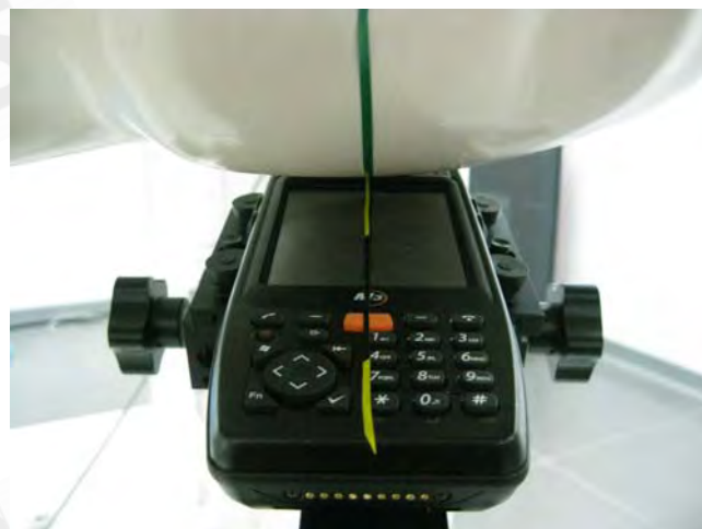
Fig.6 Left Head Section / Ear-Tilt Position(15°)
