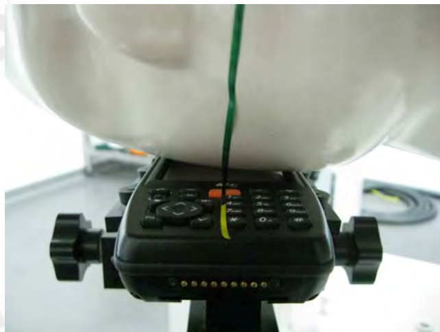
Fig.3 Right Head Section / Cheek-Touch Position
