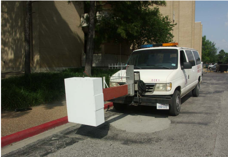
Figure 1-2 GPR system mounted on a vehicle for measurements
