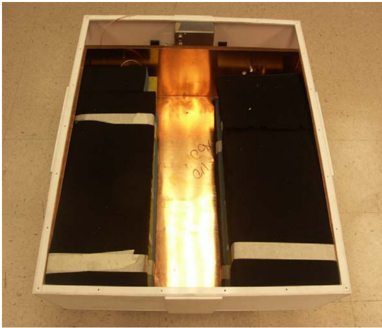
Figure 81 TEM horn antennas installed in the box
