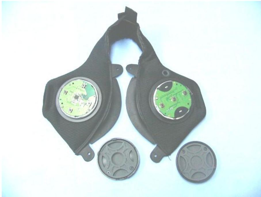
Main & RF board component side
