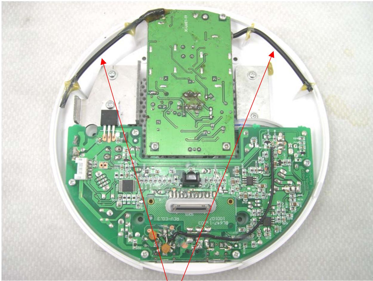
Length of the antenna wire 8.5cm each,  $\Phi = 3.0\text{mm}$
