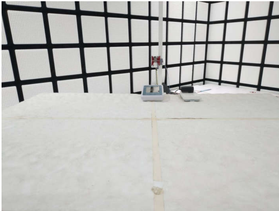
Radiated spurious emission Test Setup-2(Above 1GHz)
