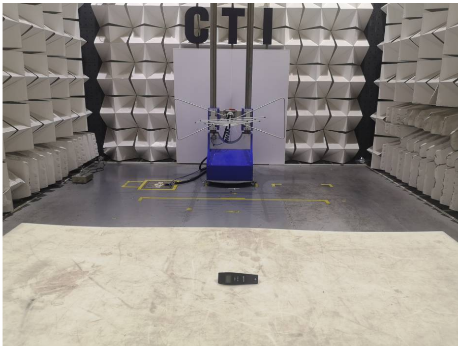
Radiated spurious emission Test Setup-2(Below 1GHz)
