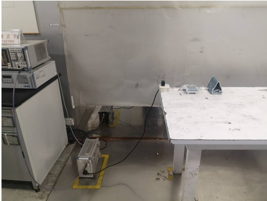
Conducted Emissions Test Setup
