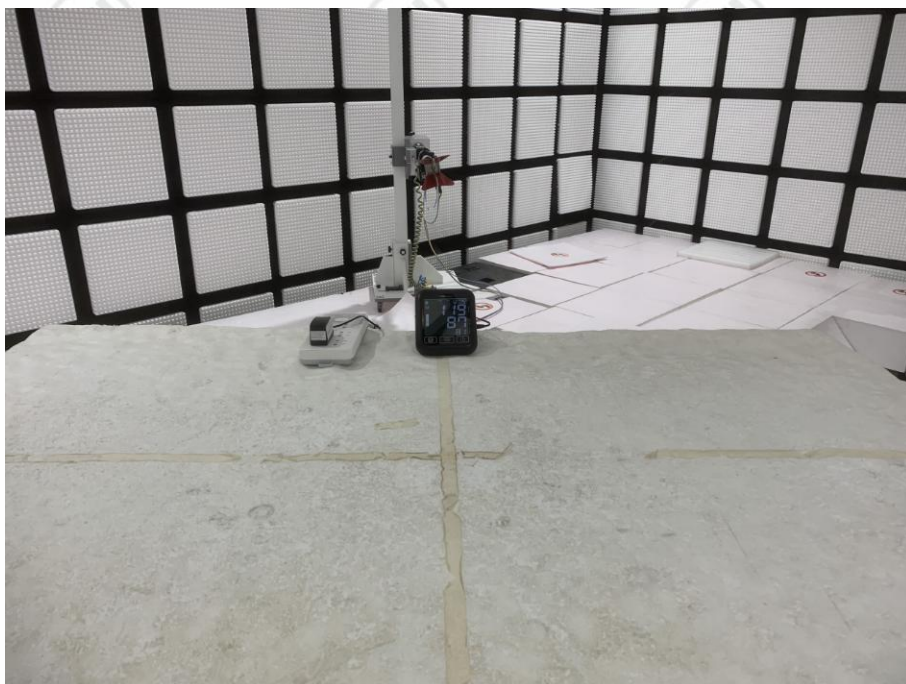
Radiated spurious emission Test Setup-2(Above 1GHz)
