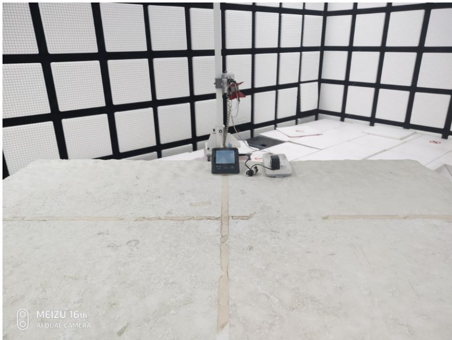
Radiated spurious emission Test Setup-2(Above 1GHz)
