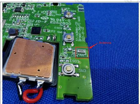
The antenna is Metal antenna. The best case gain of the antenna is 0dBi. From the PCB antenna lead of the module to the metal antenna on the other side of the board.
