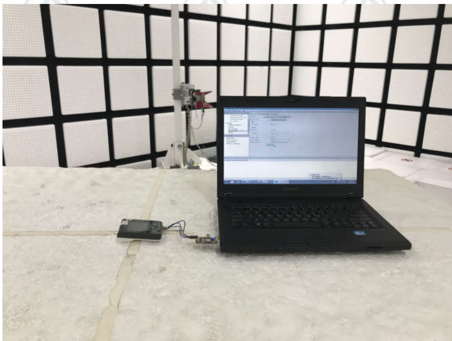
Radiated spurious emission Test Setup-2(Above 1GHz)
