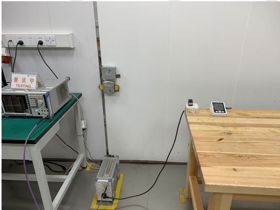
AC Power Line Conducted Emission
