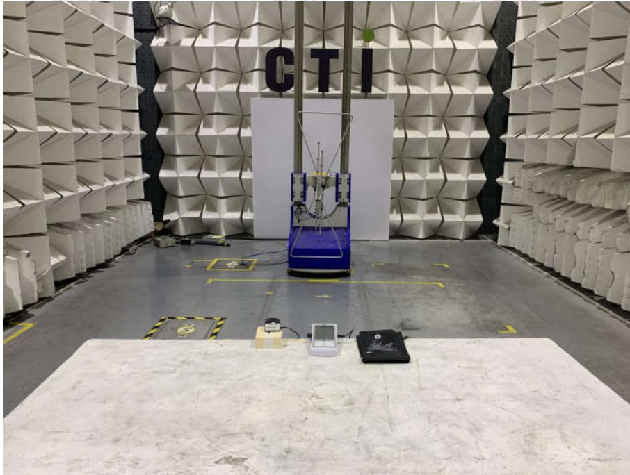
Radiated spurious emission Test Setup-1(Below 1GHz)
