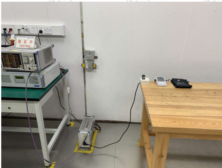
Conducted Emissions Test Setup
