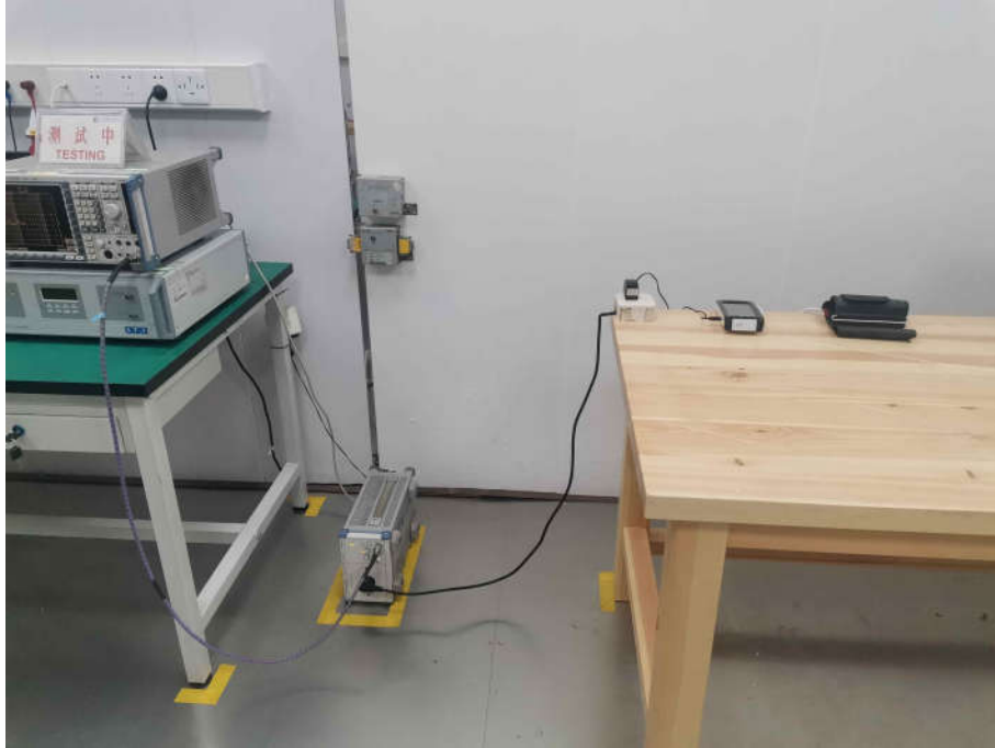
Conducted Emissions Test Setup
