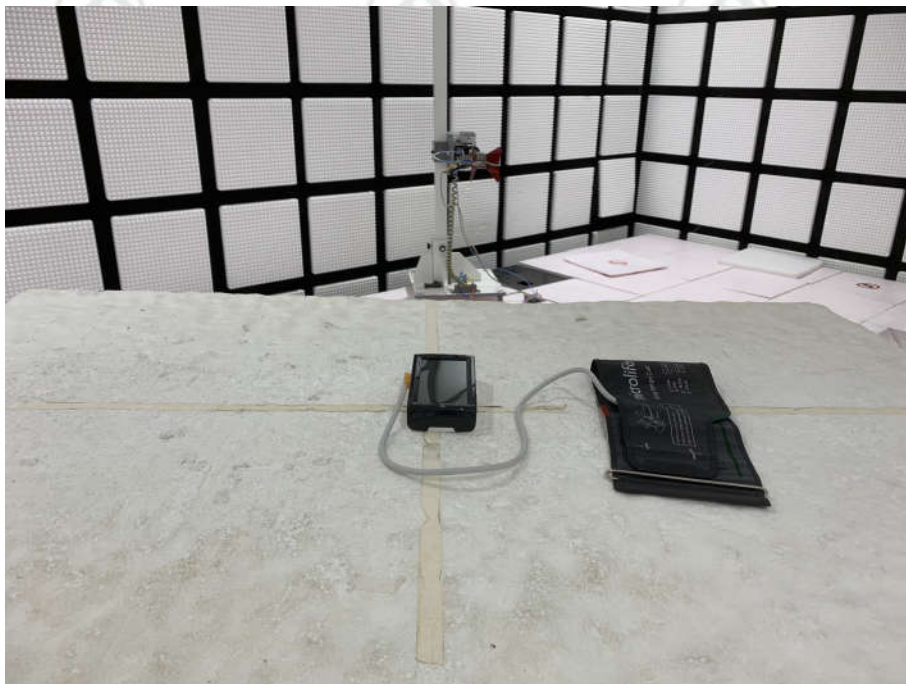
Radiated spurious emission Test Setup-2(Above 1GHz)
