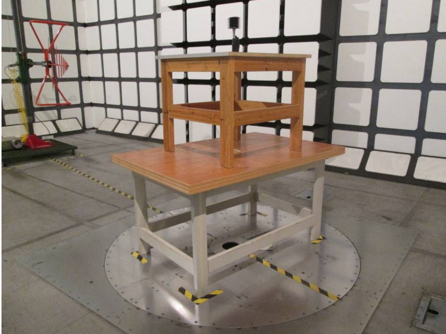
Transmitting Radiated Emissions (Below 1 GHz)
