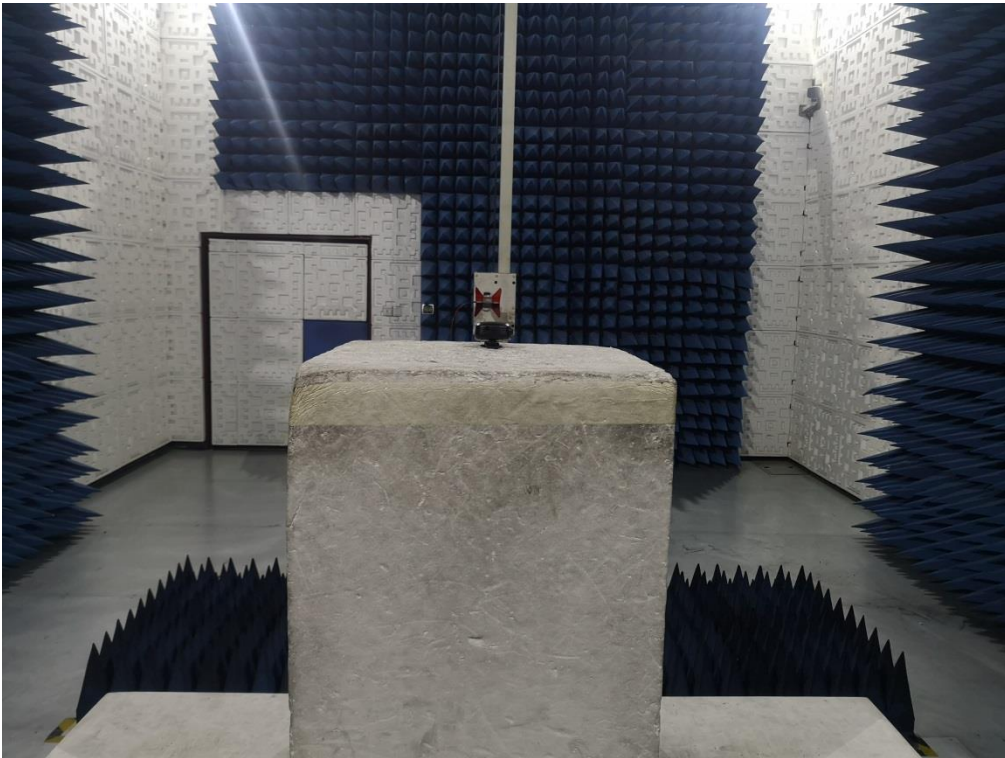
RADIATED EMISSION TEST SETUP ABOVE 1GHz
