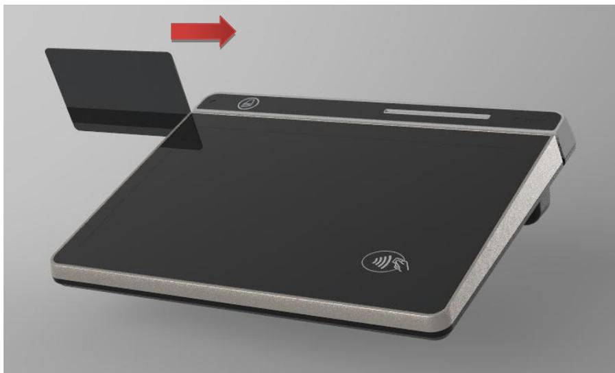
To use a IC card,the IC card chip should face the LCD.
