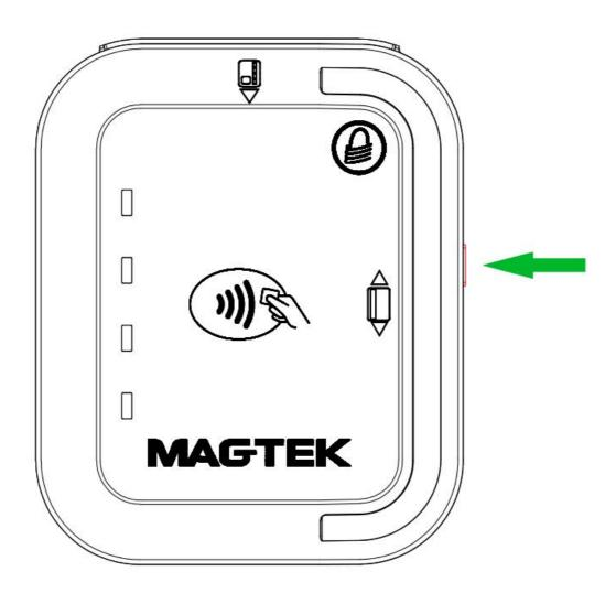
2.1.2 Second, on the card reader Connect the USB type - C interface, the other end is inserted into the host with USB interface, and then turn on power supply.
