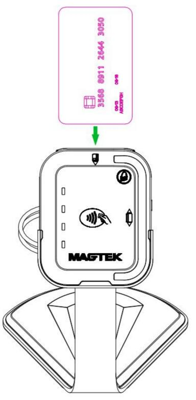
2.4 To use a NFC card Place the card near the NFC symbol on the case.
