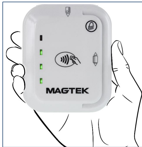
Figure 6-11 - Status LEDs Showing Battery Level
