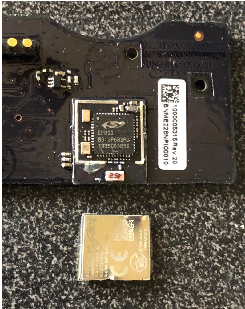
Bluetooth LE module with shield removed
