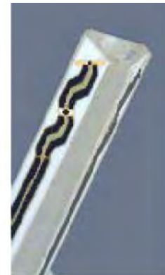
Figure 2.3 Probe Thick-Film Technique
