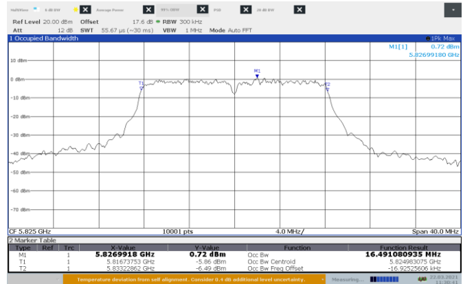
Figure 8.6-4: 99% bandwidth on 802.11a, Port B Mid Channel
