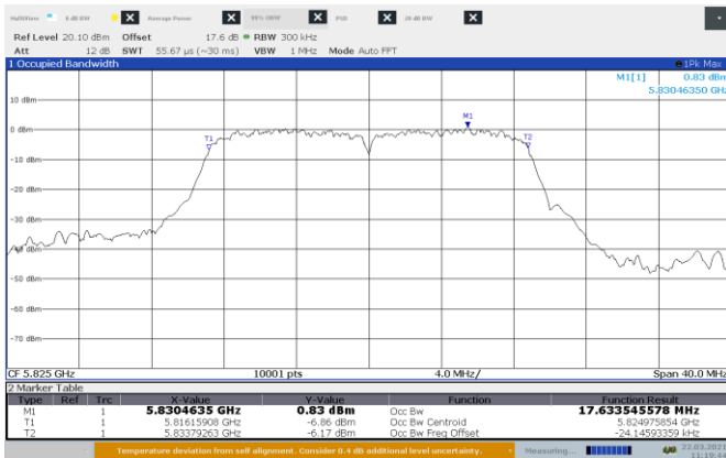
Figure 8.6-9: 99% bandwidth on 802.11ac, Port A Mid Channel
