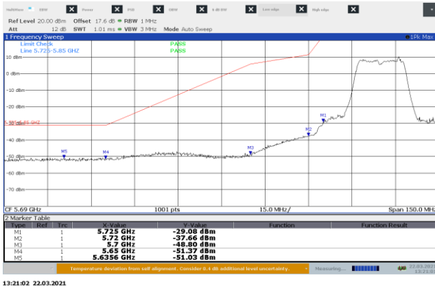
Figure 8.8-1: Conducted Lower band edge emissions, 802.11a, low channel Port A
