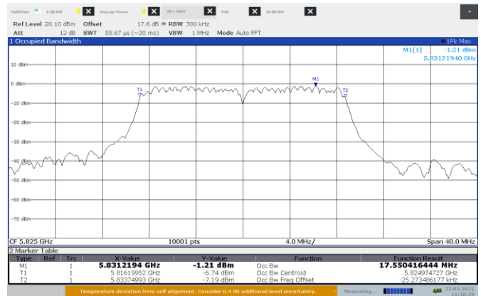
Figure 8.6-10: 99% bandwidth on 802.11ac, Port B Mid Channel
