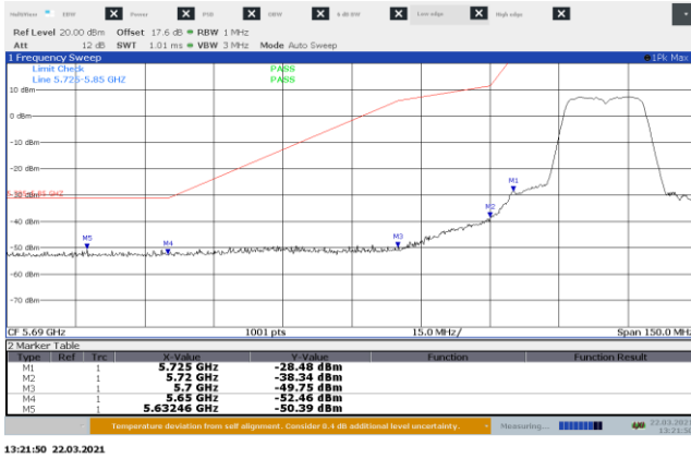
Figure 8.8-3: Conducted Lower band edge emissions, 802.11ac, low channel Port A
