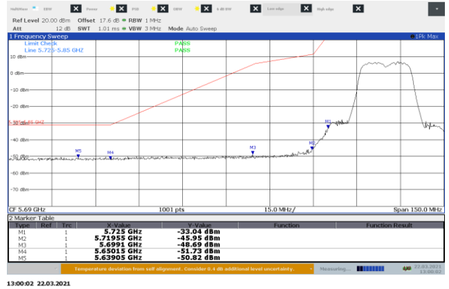
Figure 8.8-4: Conducted Lower band edge emissions, 802.11ac, low channel Port B
