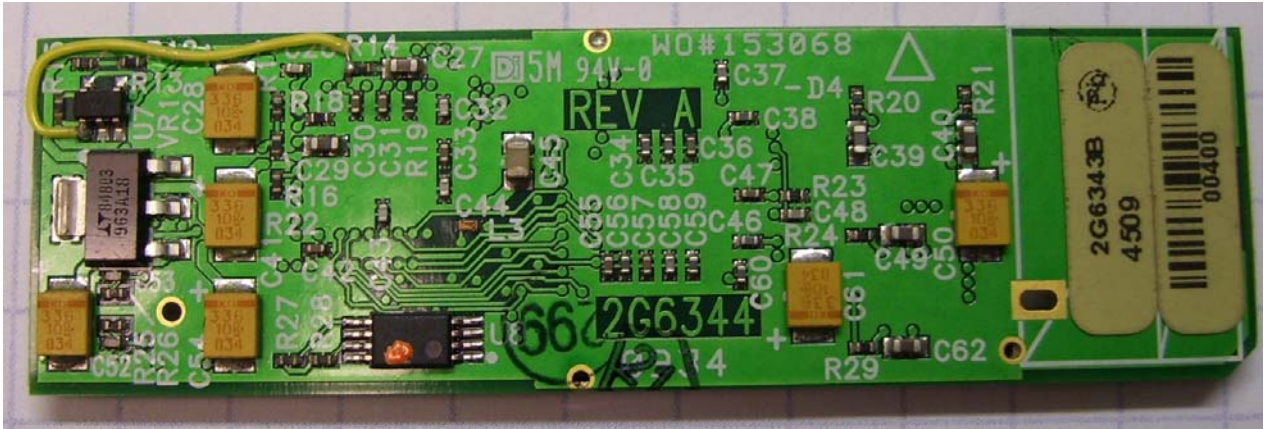
Figure 3 – Radio board only (back side)
