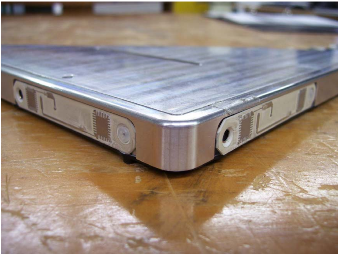
Figure 4 – Antenna(s) mounted in cassette
