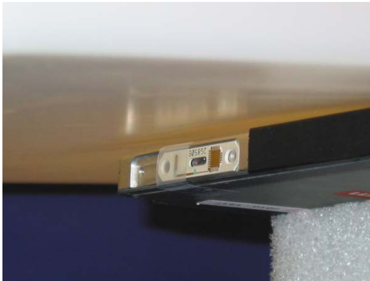
Main Antenna Bottom Of Unit Configuration
